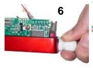
6.- Hand tighten the liquid tight fitting to establish seal.
