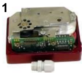
1.- Remove the liquid tight fitting from the actuator casing and insert the cable into it.
