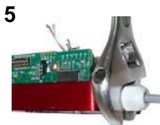
5.- Put the liquid tight fitting back and tighten (lightly with tool).
