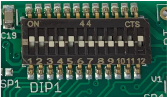
In this example DIPs 1, 2, 5 and 12 are on.
